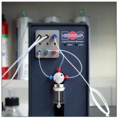
Quartz, Borosilicate Glass, PTFE, FEP, FKM, and Stainless Steel wetted surfaces ensure high chemical compatibility. CLASSIZER™ ONE measures samples at laminar constant flows of 0.2, 0.5, 1.0, 2.0, 4.0 mL/min and viscosity up to 30cS.
