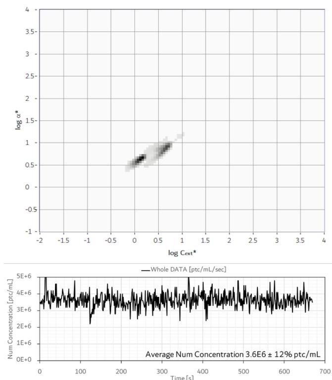
Figure 3 (top) EOS CLOUDS histogram corresponding to the whole CFA run. Two clouds are detected with different optical properties. (bottom) time evolution of the numerical particle concentration, 1 sec time resolution. The numerical concentration is stable and agrees within experimental error with expected values.
