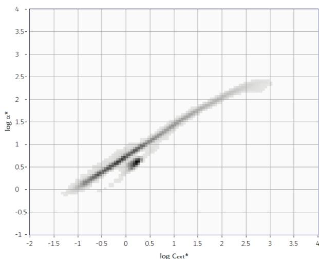
Figure 10 Merged data of two acquisitions a mix of polydisperse silicon droplets and 500nm PS spherical particles presented in Figure 9.
