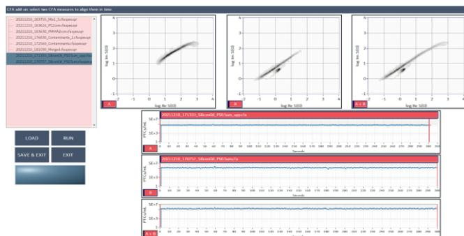
Figure 9 A screenshot of the EOS Classizer software. Two data sets are selected. The system allows to impose two zero/start points and two end points for the two acquisitions. Data of the two acquisitions are merged resulting in a third file with the merged acquisition. In this example a mix of polydisperse silicon droplets and 500nm PS spherical particles are measured in the lower and in the upper size range, then merged in one whole acquisition.
