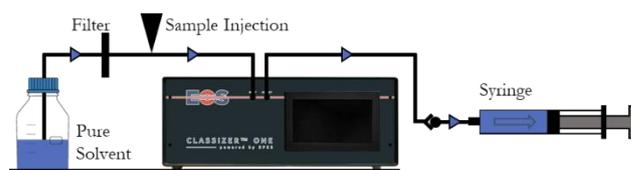
Figure 5 Simplified layout of the scheme used for this case study. A single syringe pump pulls a pure filtered solvent @ 2ccm flow. Small aliquots of samples are injected in the line through a valve.
