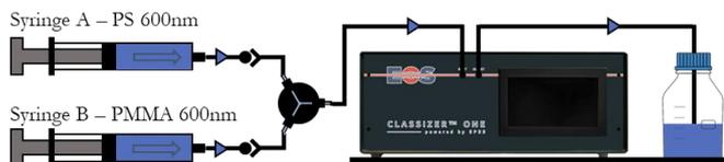
Figure 2 Simplified layout of the scheme used for this case study. Two syringes loaded with two different species of polymeric particles are pushed with an inverse time-varying velocity so the sum of the two flows is 2 mL./min. The flows are mixed, and the sample is measured using an EOS Classizer™ ONE system. In this case the sample goes to drain after the analysis, but it can be recovered for further tests if needed.
