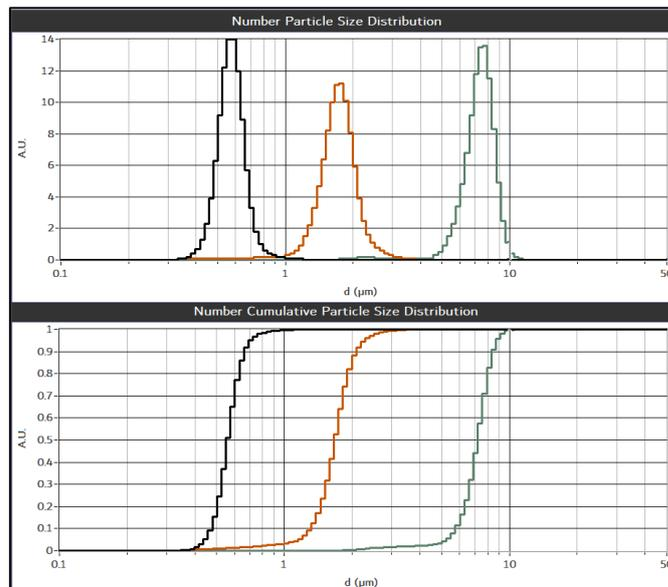
Figure 5 Numerical Particle Size Distributions and Cumulant Distributions of PMMA samples of 0.6µm, 1.8µm and 8µm diameters dispersed in filtered water. Average refractive index  $n$  is automatically calculated by EOS Classizer™ software as 1.49 @  $\lambda=640\text{nm}$ .
