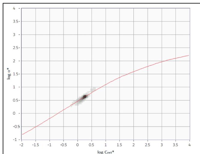
Figure 2 EOS CLOUDS histogram for a sample of PS 0.5 $\mu\text{m}$  spheres dispersed in milliQ-grade water. Position of experimental data (grey tones proportional to relative numerical concentration). Red line represents expected SPES position for PS spheres with different sizes.
