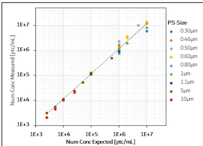
Figure 8 Estimate of the accuracy of the numerical concentration analysis of the EOS Classizer™ ONE. Polystyrene samples of different size and concentration are considered.
