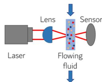
Particles are driven by a laminar fluid flow (liquid or gas depending on the application/CLASSIZER™ version) through the waist region of a tightly focused laser beam.
