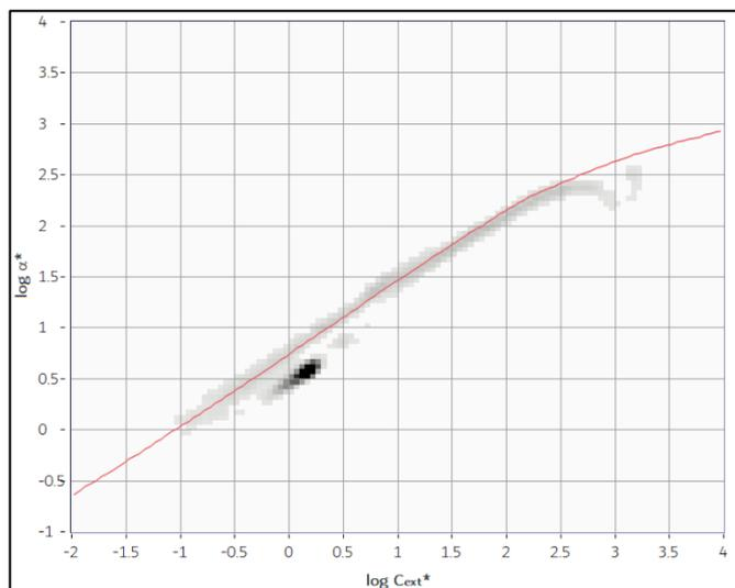
Figure 11 Example of EOS CLOUDS for a heterogeneous sample of silicon oil emulsion with polystyrene 0.5µm spheres as traceable particles. Two principal and separated populations are detected. Red line represents expected size trend for droplets of castor oil refractive index.
