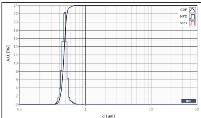
Figure 3 Experimental Numerical Particle Size Distribution of calibrated PS 0.5µm spheres dispersed in milliQ-grade water. Average particle diameter retrieved by EOS Classizer™ is 0.49 µm @ measured n=1.60.
