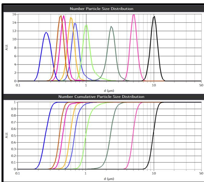
Figure 4 Numerical Particle Size Distributions and Cumulant Distributions of PS samples of 0.24µm, 0.46µm, 0.5µm, 0.6µm, 0.7µm, 1µm, 2.0µm, 5µm and 10µm diameters dispersed in milliQ water.
