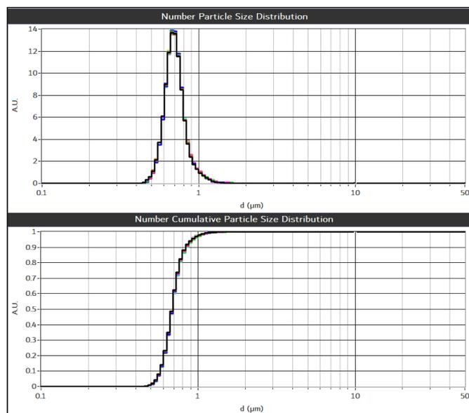
Figure 6 SPES reproducibility test. Sixteen analytical replicates of PS calibrate spheres of 0.7µm, diluted 20000 times in milliQ-grade water at 5E6 ptc/mL from an initial bulk concentration of 1E11 ptc/mL. (top) Particle Size Distribution, (down) Cumulant Particle Size Distributions.
