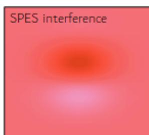
The intense transmitted beam interferes with the faint scattered wavefront in the far field, thus superimposing the two waves with the same curvature. This causes the interference pattern to exhibit intensity modulations on the spatial scale of the beam itself.
