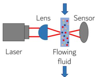
Particles are driven by a laminar fluid flow (liquid or gas depending on the application/CLASSIZER™ version) through the waist region of a tightly focused laser beam.
