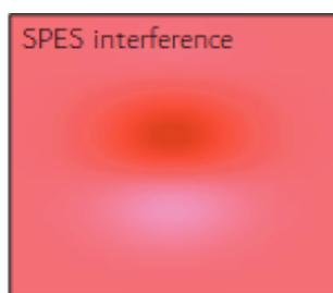
The intense transmitted beam interferes with the faint scattered wavefront in the far field, thus superimposing the two waves with the same curvature. This causes the interference pattern to exhibit intensity modulations on the spatial scale of the beam itself.
